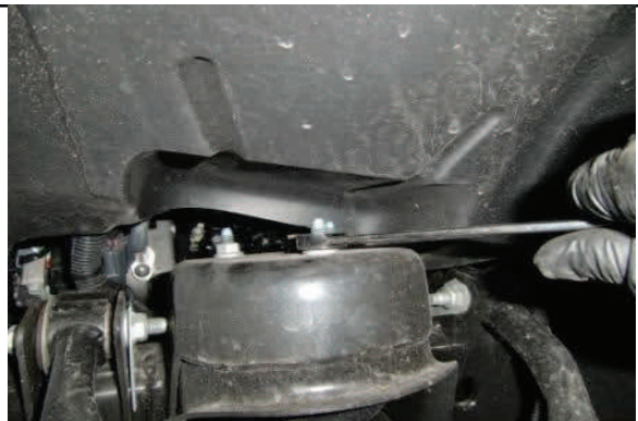
Now remove upper strut mounting nuts.
