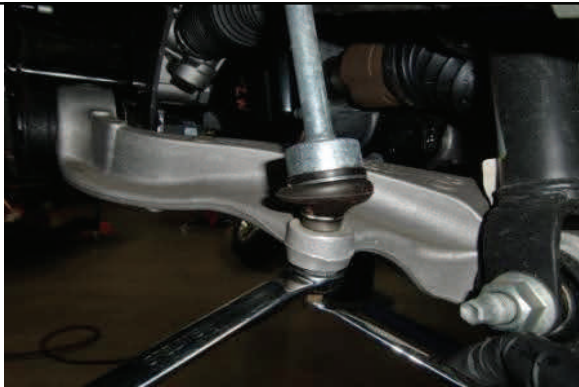
Loosen and remove lower sway bar nut.
