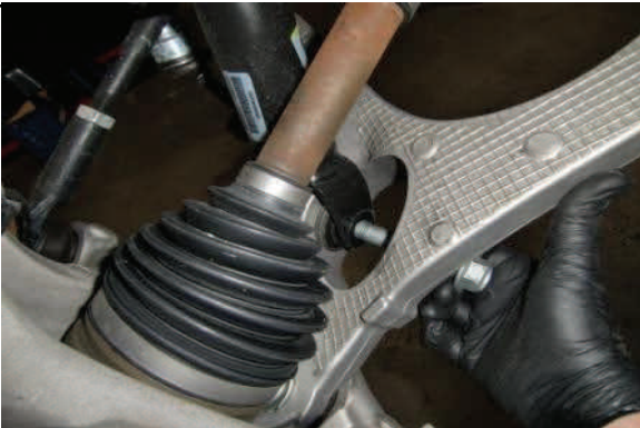
From opposite side remove bolt
