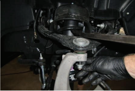
Using a pry bar, release tension, remove upper ball joint nut.
