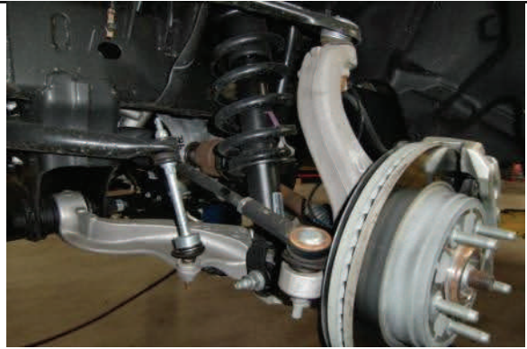
Remove front wheels and tires
