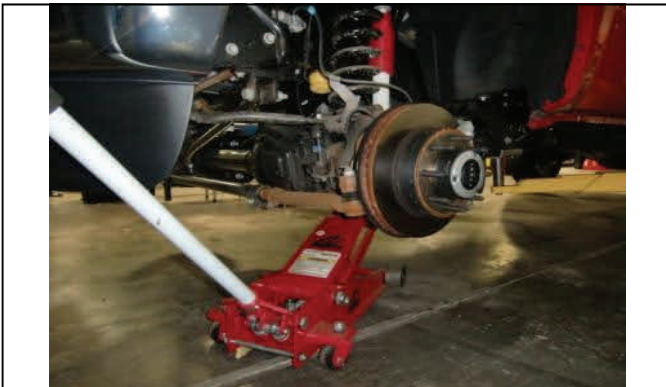
Support front axle with floor jack(s).
