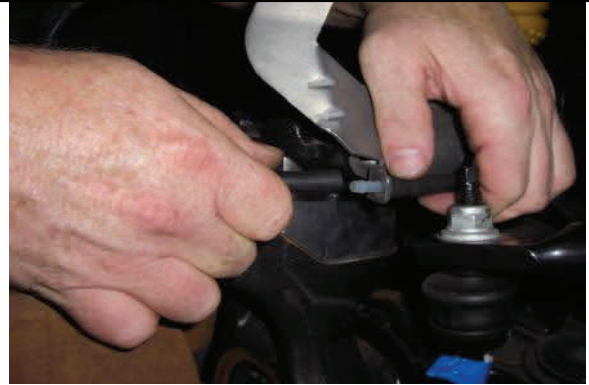
Disconnect vacuum line and clip from brake bracket
