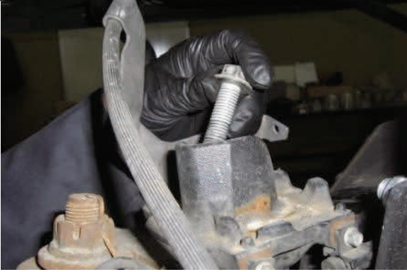
Remove bolt from middle of spring perch
