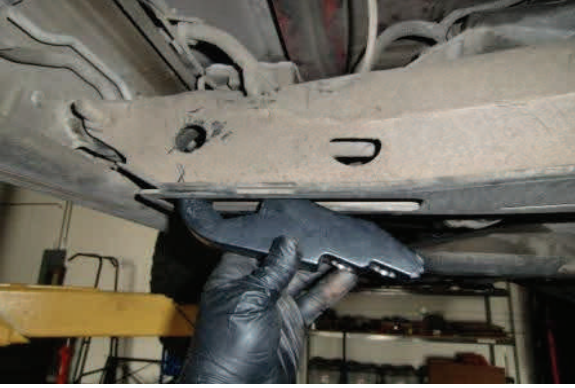
Install new ReadyLIFT forged torsion key in same position.
