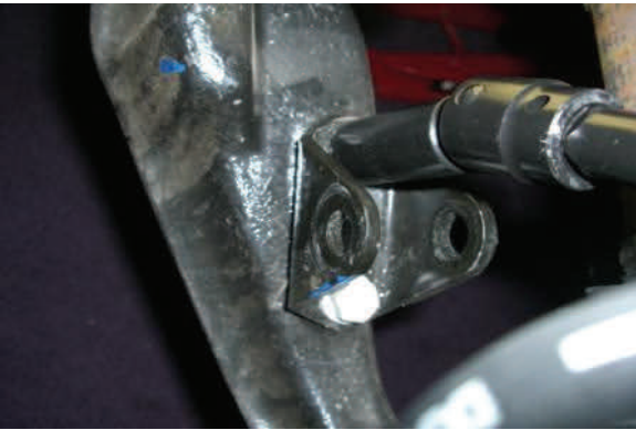
66-3050 shock extensions will replace the OE brackets
